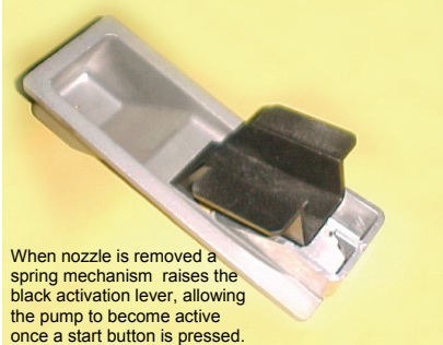
Nozzle engaged in boot forces the black activation lever into the off position.
