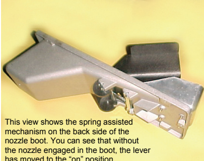
When nozzle is removed a spring mechanism raises the black activation lever, allowing the pump to become active once a start button is pressed.
