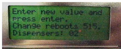
Mode 51 – Programming the number of Fueling Points
