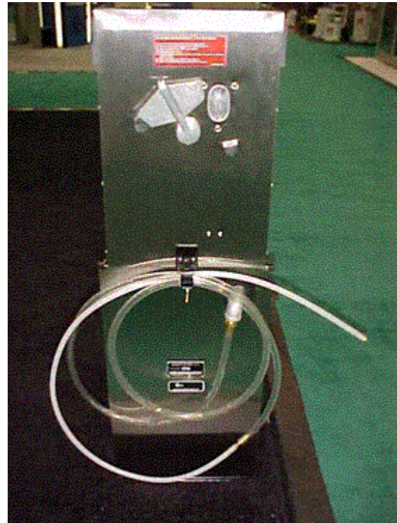
A photo of an earlier vintage DeFueler showing the Defueler hose and wand.
